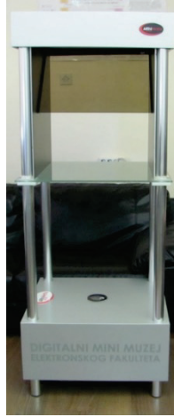
Fig. 2. Inclined projection plane device (IPPD) with two projection planes (Photo by R S. Stanković).
