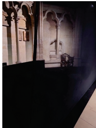
Fig. 4. Illustration of the position of mesh for a mesh projection and lighting conditions required (Photo by R. S. Stanković).
